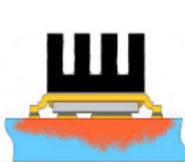
⑥ Mounted to a PCB with small clip heatsink (still air)
